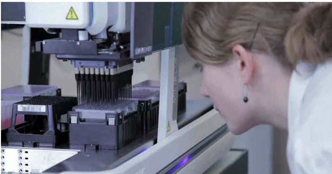
Fig. 2: Production of microtissues using a Hamilton Robotics NIMBUS system (source: InSphero AG).
